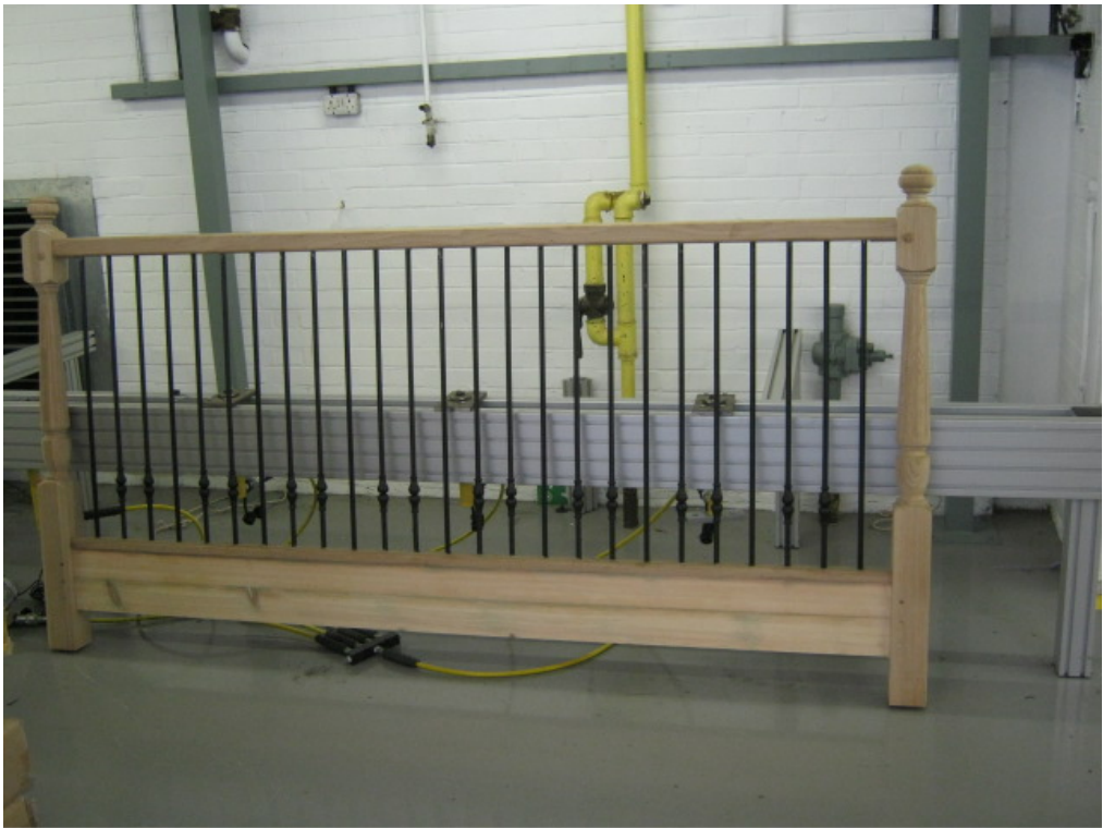
Plate 1: Metal Balusters 2.4m Horizontal Balustrade, American White Oak before Test
