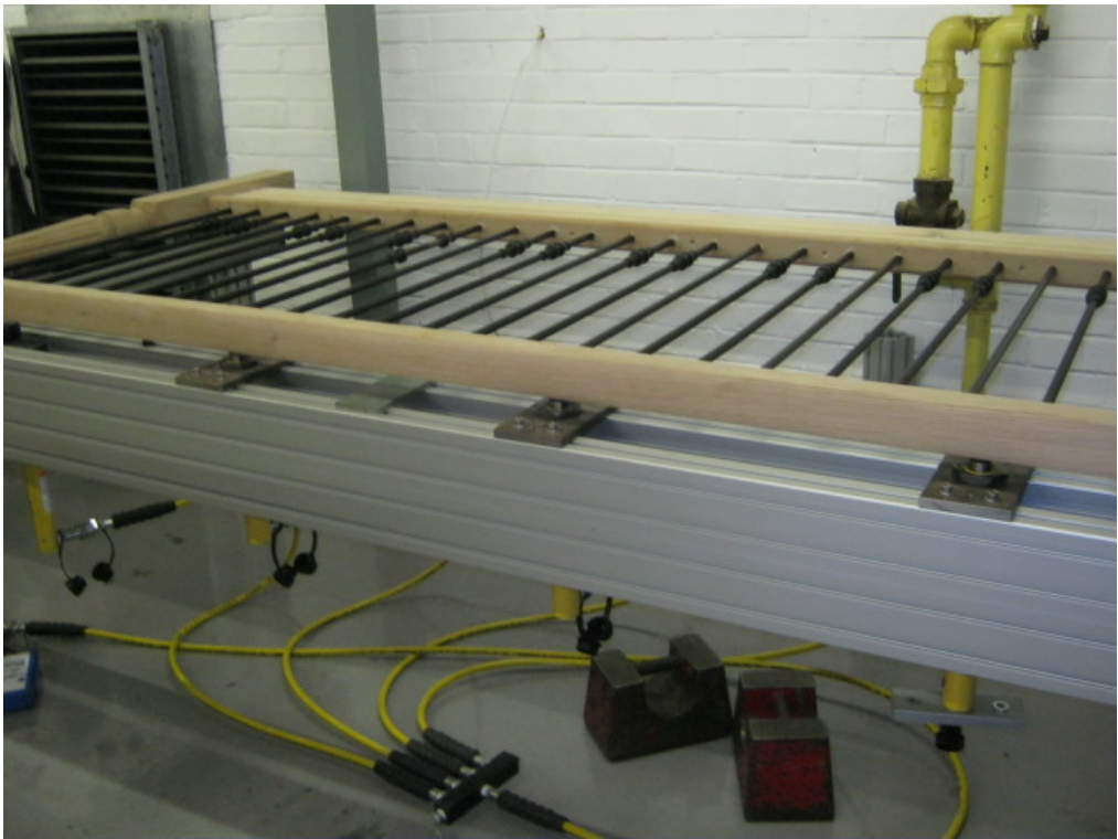
Plate 2: Metal Balusters 2.4m Horizontal Balustrade, American White Oak on Test
