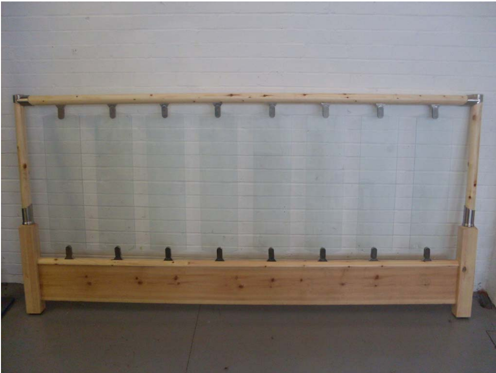
Plate 1: FUSION® Domestic Stair Unit with Glass Panels Before Test
