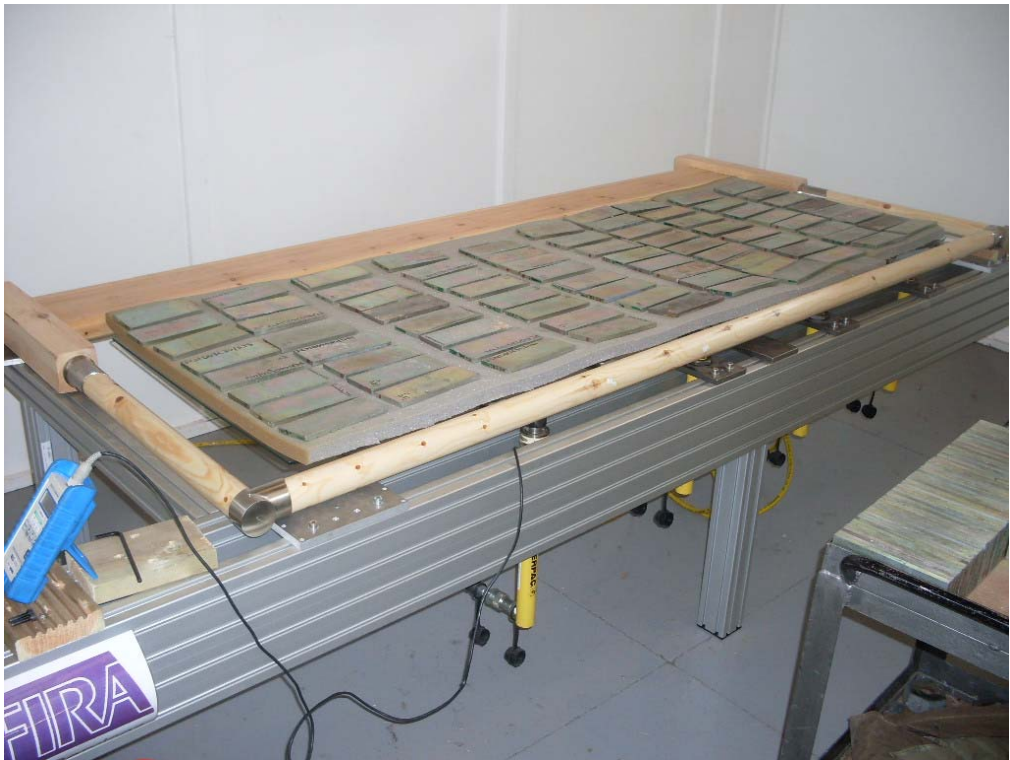
Plate 2: FUSION® Domestic Stair Unit with Glass Panels on Test
