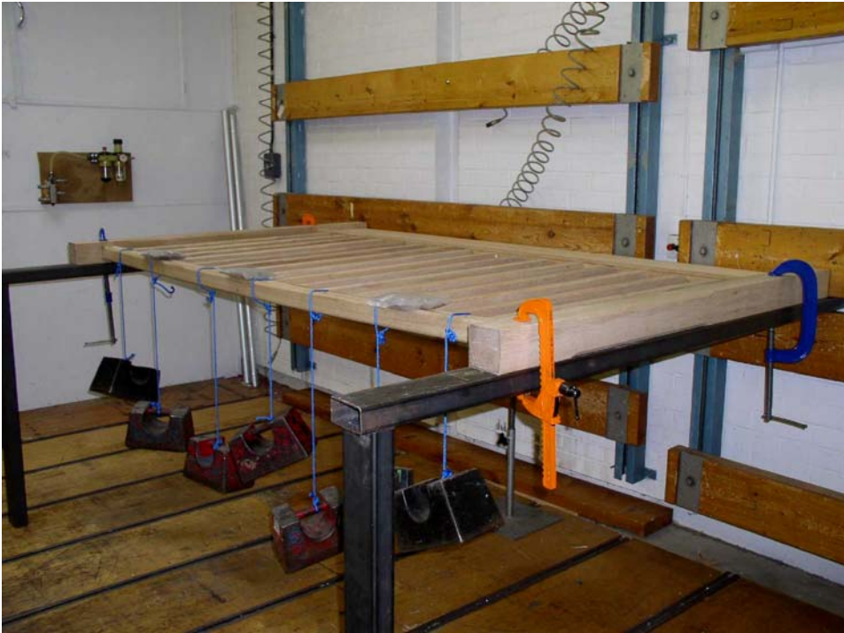
Plate 1: Landing Balustrade ref: White Oak (Euro) Stairparts, initial application of design load
