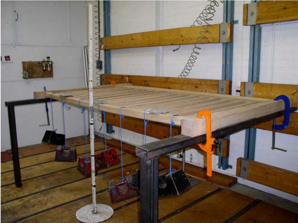
Plate 2: Landing Balustrade ref: White Oak (Euro) Stairparts, completion of application of design load
