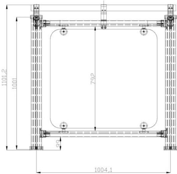
Plate 2: Drawing of Balustrade Handrail Ref: FUSION COMMERCIAL ALUMINIUM SYSTEM USING STAINLESS STEEL A4 FIXINGS with 1.2 metre long handrail and large glass infill panel
