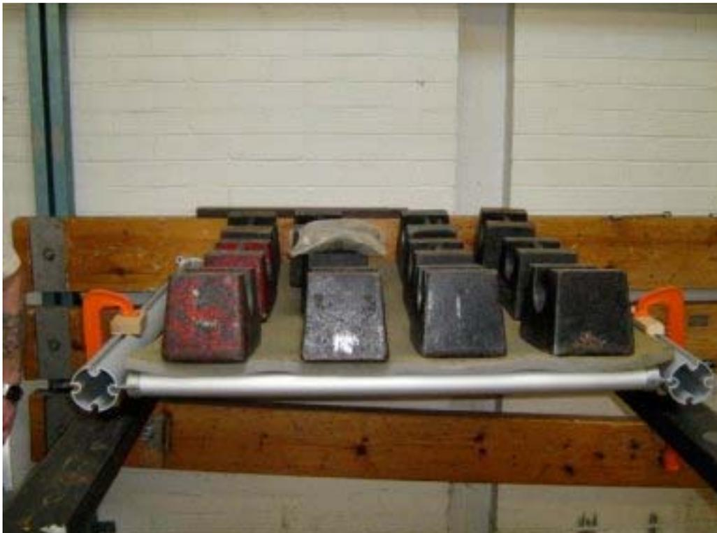
Plate 8: Balustrade Handrail Ref FUSION COMMERCIAL ALUMINIUM SYSTEM USING STAINLESS STEEL A4 FIXINGS with 1.2 – infill test
