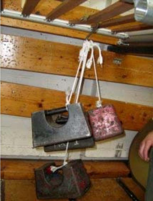
Plate 9: Balustrade Handrail Ref FUSION COMMERCIAL ALUMINIUM SYSTEM USING STAINLESS STEEL A4 FIXINGS – baluster test
