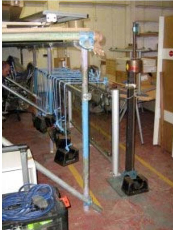
Plate 7: Balustrade Handrail Ref FUSION COMMERCIAL ALUMINIUM SYSTEM USING STAINLESS STEEL A4 FIXINGS - on test
