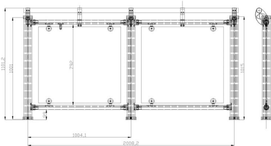
Plate 1: Drawing of Balustrade Handrail Ref: FUSION COMMERCIAL ALUMINIUM SYSTEM USING STAINLESS STEEL A4 FIXINGS with 2.2 metre long handrail and large glass infill Panel
