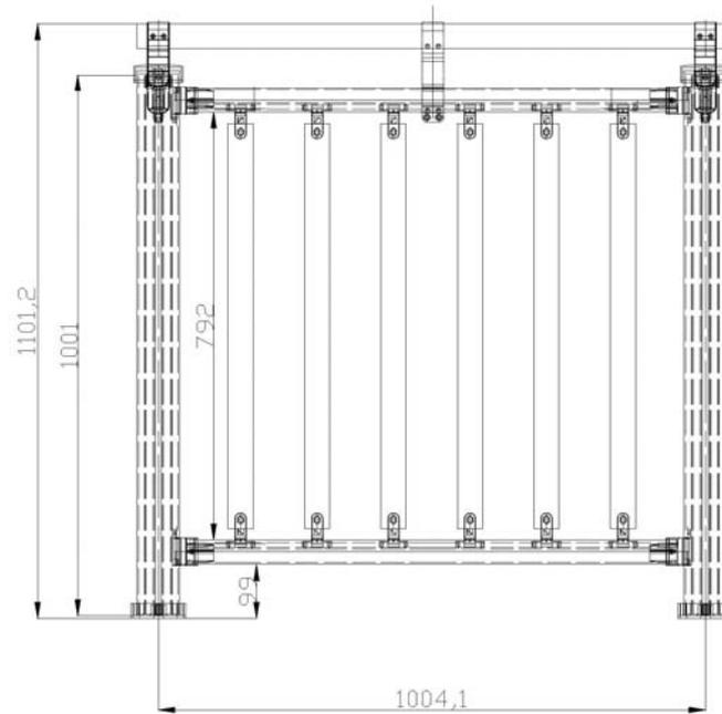
Plate 5: Drawing of Balustrade Handrail Ref: FUSION COMMERCIAL ALUMINIUM SYSTEM USING STAINLESS STEEL A4 FIXINGS with 1.2 metre long handrail and hardwood balusters
