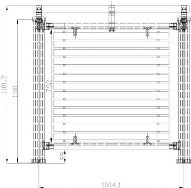
Plate 4: Drawing of Balustrade Handrail Ref: FUSION COMMERCIAL ALUMINIUM SYSTEM USING STAINLESS STEEL A4 FIXINGS with 1.2 metre long handrail and slatted hardwood infill panel
