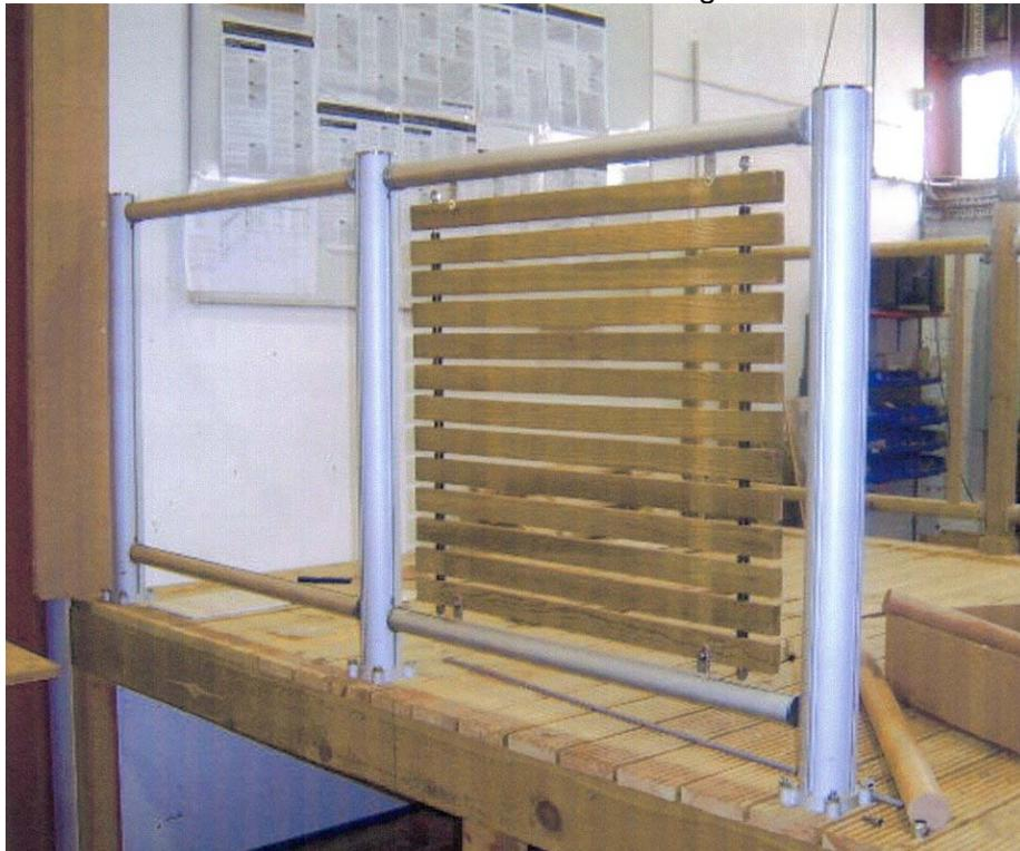
Plate 6: Balustrade Handrail Ref FUSION COMMERCIAL ALUMINIUM SYSTEM USING STAINLESS STEEL A4 FIXINGS
