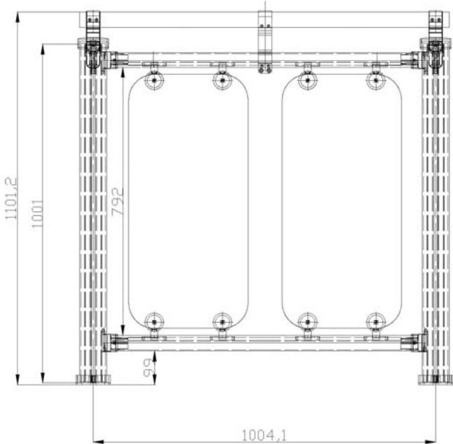
Plate 3: Drawing of Balustrade Handrail Ref: FUSION COMMERCIAL ALUMINIUM SYSTEM USING STAINLESS STEEL A4 FIXINGS with 1.2 metre long handrail and small glass infill panels
