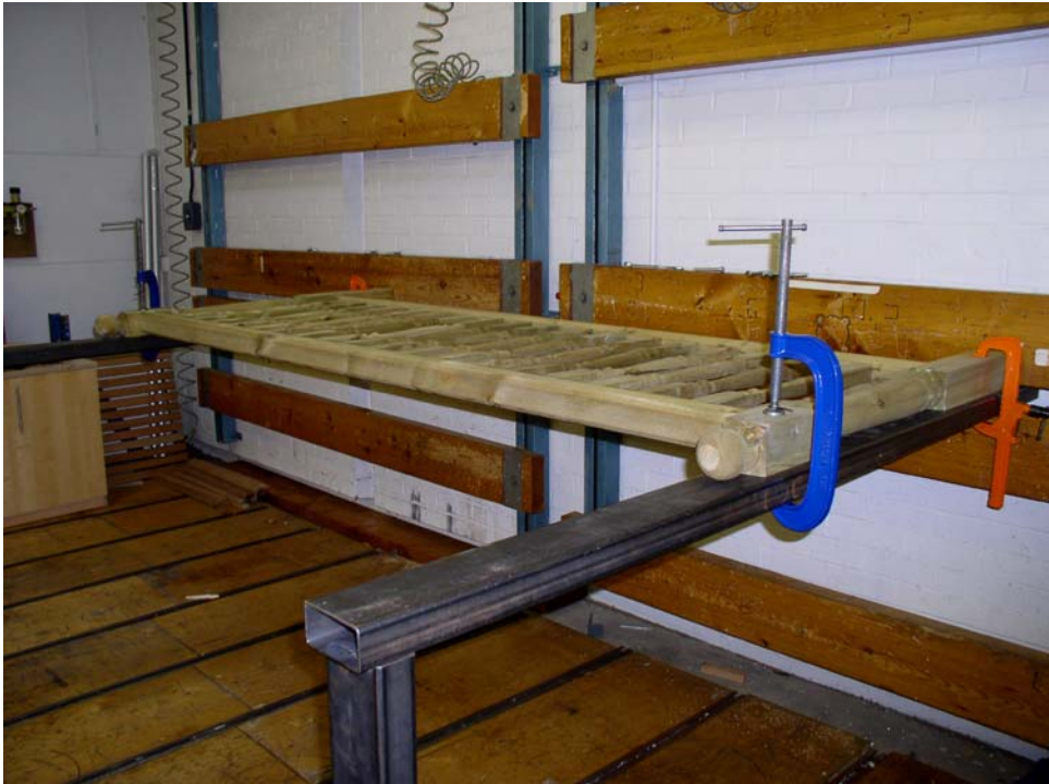
Plate 1: Decking Balustrade ref: New Fixing Bracket (1800mm), before test
