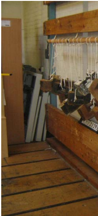
Plate 2: Commercial Fusion Handrail loaded for heavy commercial test.
