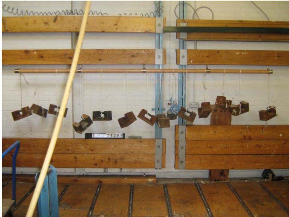
Plate 1: Commercial Fusion Handrail loaded for light commercial test
