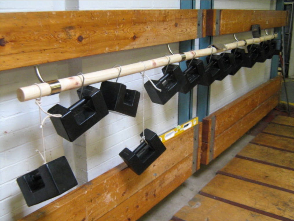
Plate 4: Loaded Handrail to 0.74kN/m
