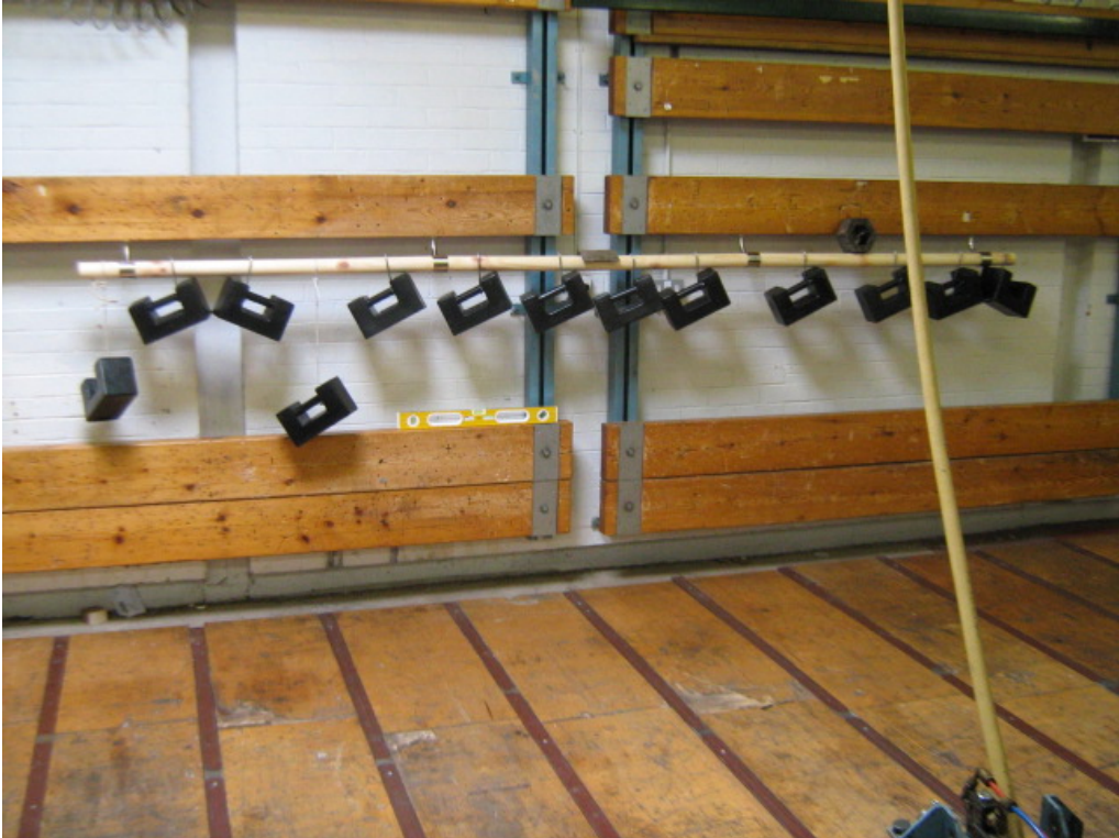
Plate 5: Handrail Loaded to 0.74kN/m
