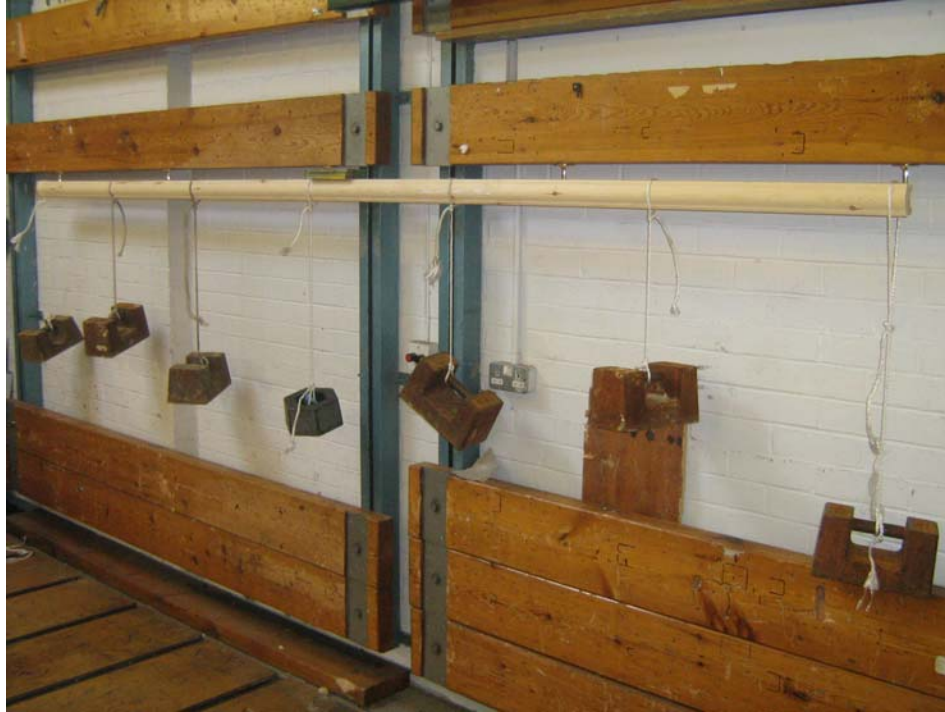
Plate 1: Domestic Light Handrail loaded at 0.36kN/m
