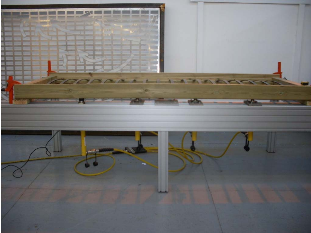
Plate 2: OB12 Metal Baluster Unit on Test
