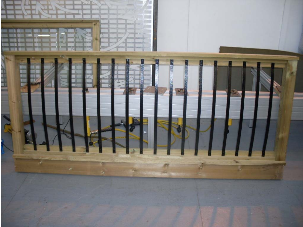
Plate 1: OB12 Metal Baluster Unit before Test
