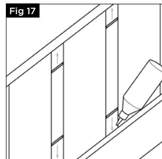
Cut all fillets to calculated length and correct angle (Fig 14). Apply bead of clear silicone to both handrail and baserail grooves ensuring you also put a bead on side wall of handrail groove. The silicone will act as an adhesive but also stop the potential movement of the glass panels over time.
