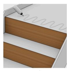
**Step 4** – apply an even/generous bead of polymer adhesive to the topmost tread. Mark and cut the tread to the correct size and lay onto the polymer adhesive.
