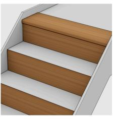
**Step 5** - Apply and even/firm pressure, making sure the tread nosing laps correctly over the riser, applying additional weights onto the top face of the tread may help.
