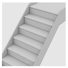
**Step 1** – before you begin, remove all floor covering, make sure that all step/riser surfaces are even and no surface defects, these can be sanded if needed, all surfaces should be clean and dry.
