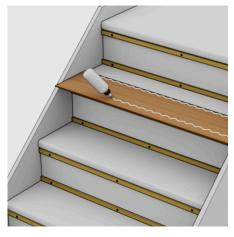
**Step 3** - cut two richard Burbidge risers to the correct sizes, glue these into place onto the packing battens...
