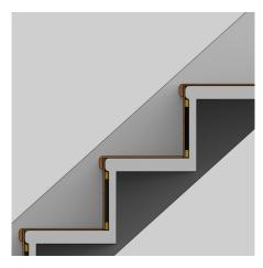
This is the side view of the installation of the tread/riser kit. When you have chosen the flooring that you intend to install on the top landing you should purchase the appropriate threshold to bridge the join between the two surfaces, if you are installing carpet you may chose to glue/pin this over the top and around the nosing for a neat finish.
