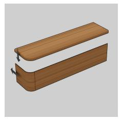
You can then offer this up to work out where the tread will rest on top of the riser. Trim the tread to fit the width and the back face of the tread to the correct depth (you may need to trim to affix around the newel post as well).
