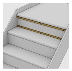
**Step 2** – prepare your timber battens, cut these to the width of the tread and screw into position.
